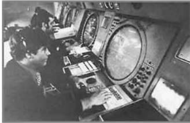
Automated Radar Traffic (ARTS) System at Jacksonville Center circa 1970. (Source: FAA)
